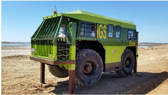
Figure 3. Typical in-situ testing and sampling rig
