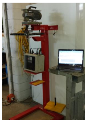
Figure 7 – A Vane Shear Test Apparatus Under Calibration Using Dead Weights
