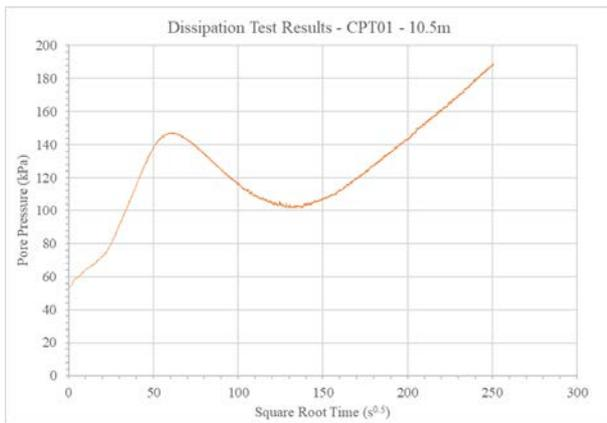
Figure 6b. Location 1 - Dissipation in Root Time, using Silicone Oil.
