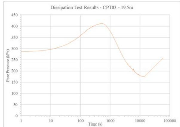
Figure 8a. Location 3 - Dissipation in Log Time, using Silicone Oil.
