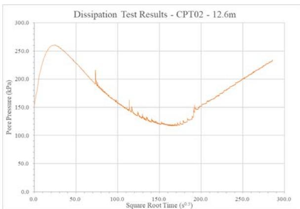
Figure 7b. Location 2 - Dissipation in Root Time, using Silicone Oil.
