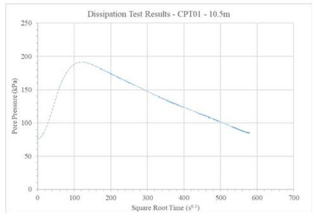
Figure 5b. Typical Dissipation Test Results in Root Time.
