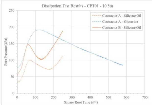
Figure 9. Dissipation Test Results at Location 1 (in Root Time).
