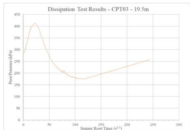
Figure 8b. Location 3 - Dissipation in Root Time, using Silicone Oil.
