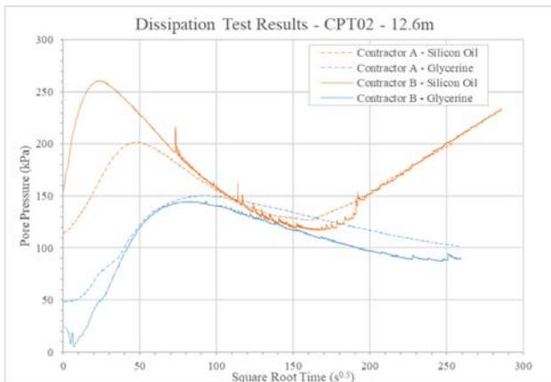
Figure 10. Dissipation Test Results at Location 2 (in Root Time).
