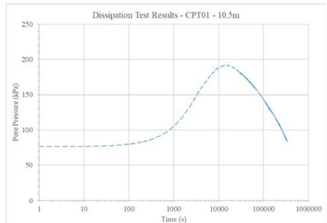
Figure 5a. Typical Dissipation Test Results in Log Time.
