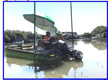
Piezocone and DMT testing in very shallow swamps, creeks, dams and lakes is now possible using IGS's "Punt Rig".
