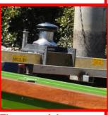
The powerful recovery winch can pull the Punt Rig around and out of the mud/slime.
