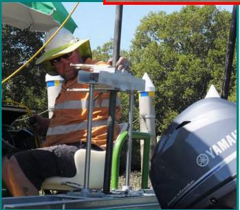
Push capacity is 8kN which is plenty for soft clays and tailings materials.
