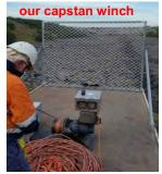
The outcome: a number of CPTu tests were successfully done to depths up to 25m and pore pressure dissipation tests were run
