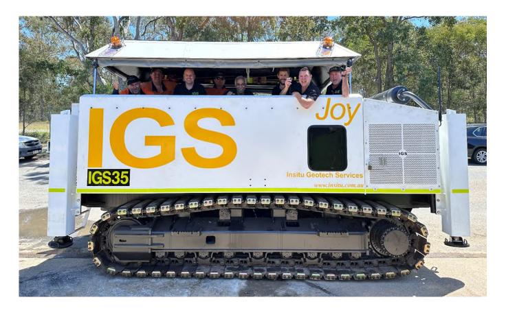
IGS35 "Joy" is has the highest push capacity of the IGS fleet of custom designed in situ testing and sampling rigs. Australian designed and manufactured the standard operating weight of this rig is 17.8t, however, if fully ballasted, the full 400kN (40t) push capacity can be mobilised. Truly a formidable and versatile rig ready to meet the challenges of your project.
