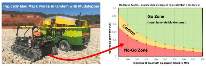
Mudskipper can CPT probe to prove-up access for Mad Mack - provides safe and defensible access system on extremely soft sites
