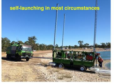
Purpose-built mini-jack-up rig Transportable on our flat-top truck Self-unloading & self-launching Overall length ~5.5m Width 3.8m Twin pushers - less set-ups needed Minimum mass ~6.5t unballasted Maximum mass ~10.5t water-ballasted Pusher capacity 150kN Suction feet add extra push reaction High Accuracy GNSS GPS on board
