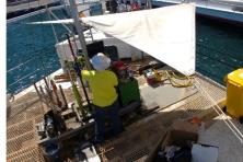
Multi-purpose rig on sled with own winch – can self-winch to locations
